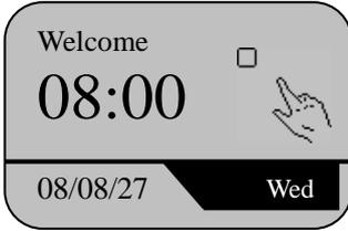
Perform validation according to preset modes (e.g. fingerprint, password, sensor card No. or combination).
